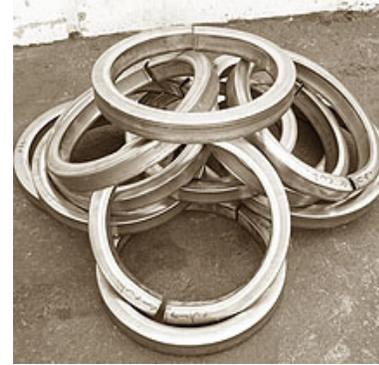
Rolled Stainless Steel Tube Rings
