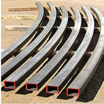
Rectangular Tube Rolled Hardway
