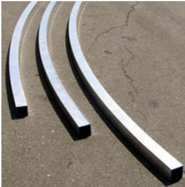
Pipe Rolling and Tube Rolling Aluminum square tube rolled
