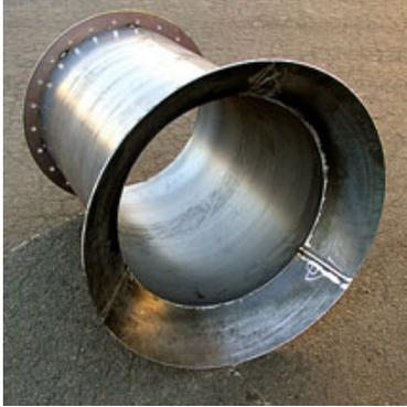
Rolled Cylinder Welded and Punched
